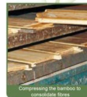
Compressing the bamboo to consolidate fibres
